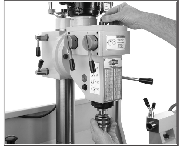
Figure 45. Aligning drawbar with chuck arbor.
